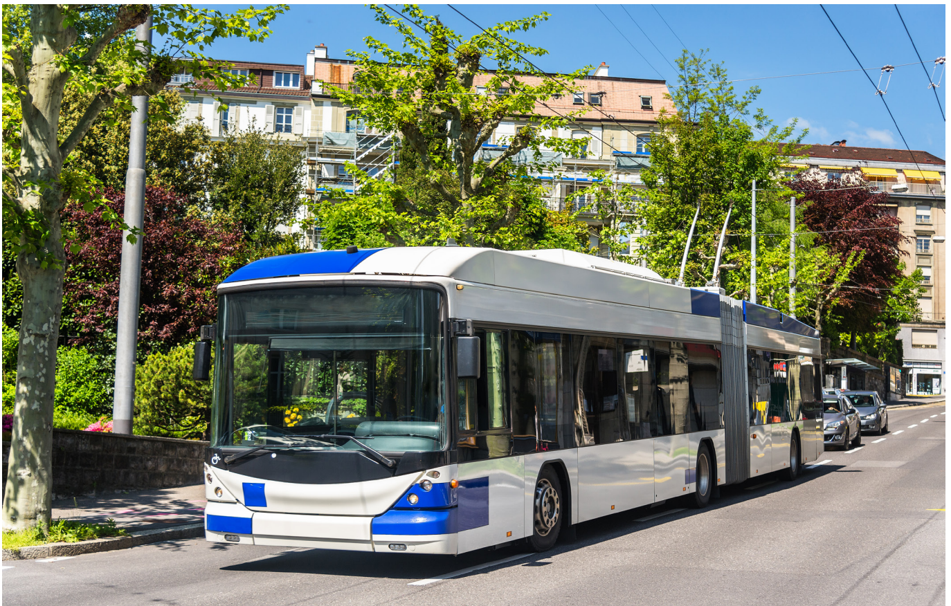
— Trolley-buses which can operate with both catenaries and batteries are becoming more common.
